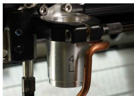
Lens 4.0" Thick cutting and fast engraving
