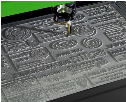
Engraving & laser cutting of custom ink stamps
